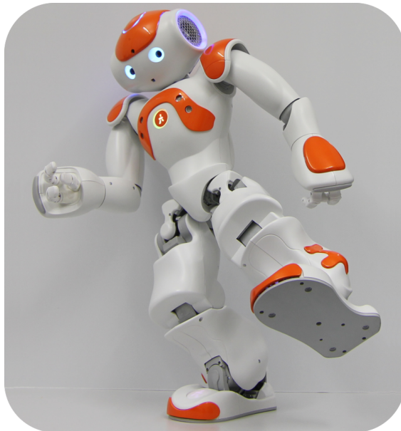
Fig. 1: A NAO robot learns to lift up one leg and stay balanced using a novel latent space policy search method. The co-articulation of the joints, needed for successful execution of the motor skill, is represented in the low-dimensional latent space.
